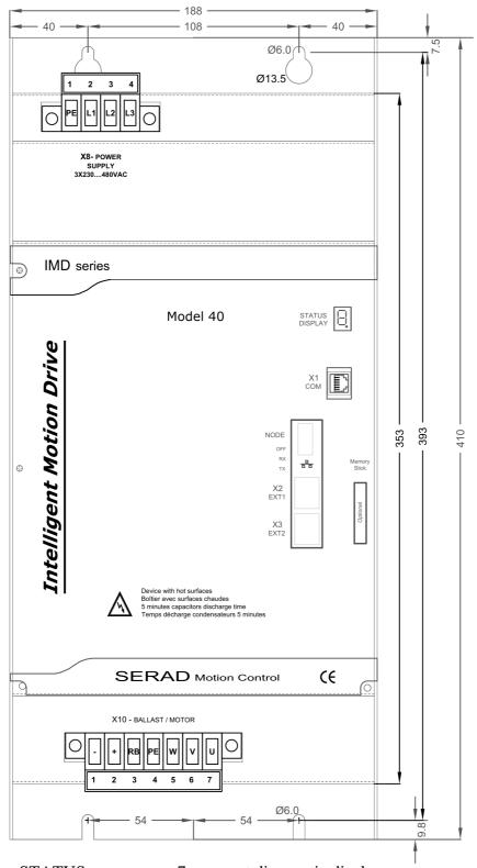
**STATUS** 7-segment diagnostic display RS-232 serial port for communication with a PC X1 COM EXT1 X2 Extension: Optional communications ports X3 EXT2 Extension: Optional communications ports X8 **POWER SUPPLY** Single / Three-phase power supply X10 RB / MOTOR External braking resistor and motor supply
