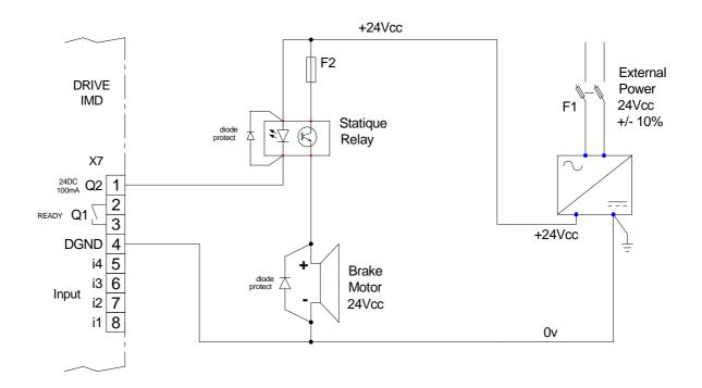
The output Q2 is NPN open collector, 100mA max. The load must be connected between Q2 and +24Vdc.
